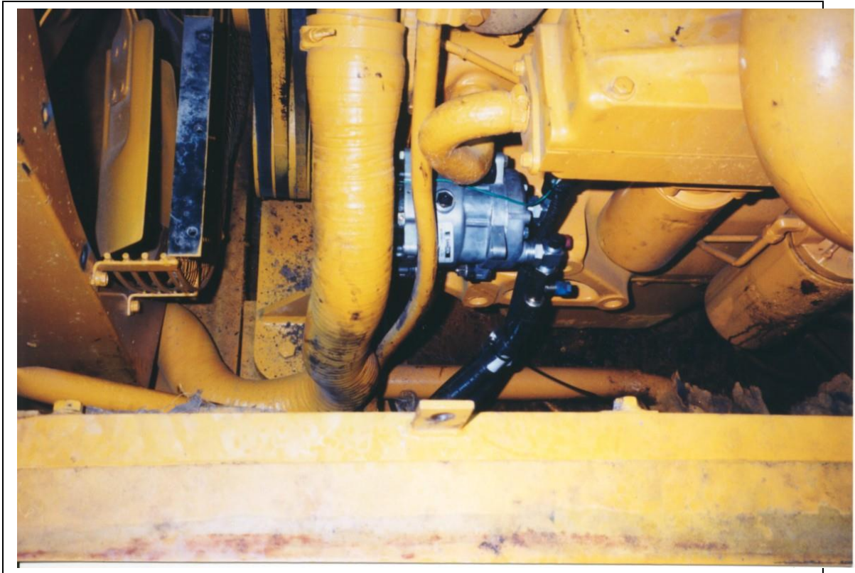
Compressor and mount in place on engine. View from top side of engine compartment.
